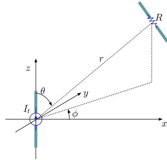
**Current  $I_r$  that flows through the resistor  $R$  connected across the antenna terminals is induced by the tangential components of incident wave fields on the conducting arms of the dipole antenna; this response is a straightforward consequence of the need to maintain tangential boundary conditions on the antenna surface.**
