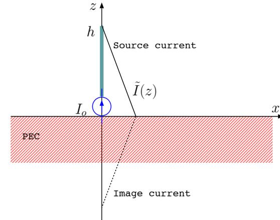
of a two-wire dipole of length  $L = 2h$  (on which the condition is satisfied *ipso facto*),
