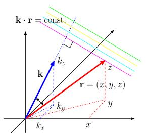
The propagation direction is specified by the unit vector  $\hat{k} = \frac{\mathbf{k}}{k} = \frac{3\pi\hat{x} - 4\pi\hat{y}}{5\pi} = 0.6\hat{x} - 0.8\hat{y}.$ The wavelength is
