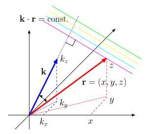
• In a homogeneous region where  $\epsilon$ ,  $\mu$ , and  $\sigma$  are, by definition, independent of **r**, plane-wave solutions of phasor-form Maxwell's equations given in the margin become possible provided that
