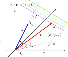
We have obtained these vector-algebraic relations from phasor-form Maxwell's equations in the margin after replacing the vector-differential operator  $\nabla$  by the vector-algebraic operator  $-j\mathbf{k}$ .
