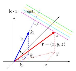
• The general case with non-zero components  $(k_x, k_y, k_z)$  corresponds to a plane wave propagating in the direction of unit vector
