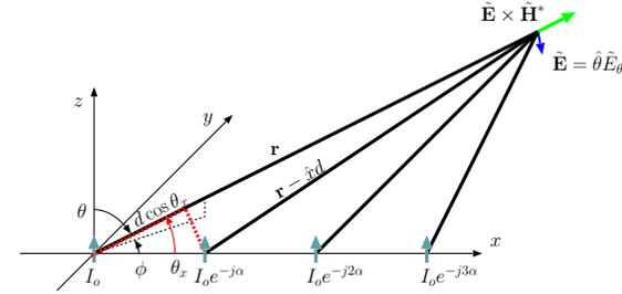
**Designing the feed network:** The required phase delays
