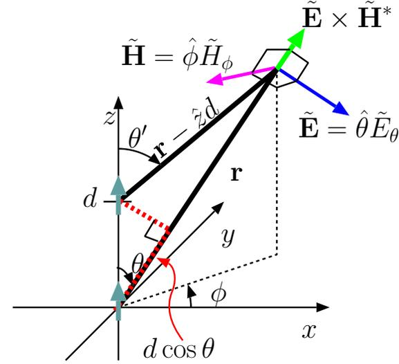
**Example 3:** For the two-element antenna array of short dipoles examined in Examples 1 and 2 with field phasor
