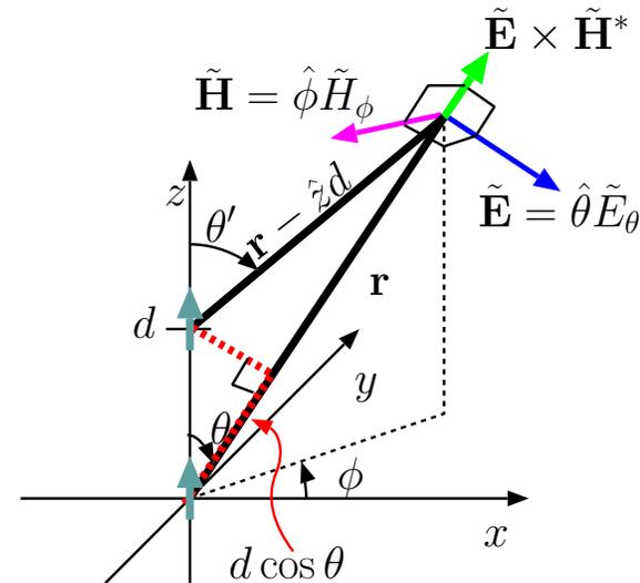
**Example 1:** Two  $\hat{z}$  polarized dipole antennas with equal input currents  $I_o$  are located at  $(0, 0, 0)$  and  $(0, 0, d)$ . Find the phasor expression  $\tilde{\mathbf{E}}(\mathbf{r})$  representing the superposition of the fields radiated by each dipole individually. What are the maximum and minimum values of the field intensity  $|\tilde{\mathbf{E}}(\mathbf{r})|$  as compared to intensity  $|\tilde{\mathbf{E}}_1(\mathbf{r})|$  of the field due to the dipole at the origin?
