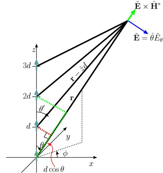
The same interference principle governs  $N$ -element arrays: at locations where field phasors from individual elements have the same angle, constructive interference takes place, and the radiation field of the array is strong. At other locations where field phasors from individual elements cancel one another, the field of the whole array is weak.
