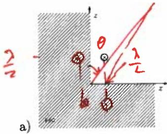
Consider a  $\hat{y}$  polarized short dipole antenna located at  $(x, y, z) = (\lambda/4, 0, \lambda/8)$  next to a PEC corner reflector as shown in the diagram depicted on the left. The dipole is indicated by the "tail view" of an arrow pointing in  $+y$  direction.
