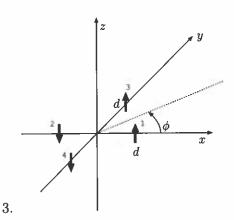
Consider the four-element array of identical  $\hat{z}$ -polarized Hertzian dipoles placed at a distance d away from the origin on  $\pm x$  and  $\pm y$  axes as depicted on the left. All four dipoles are driven by identical input currents in the reference directions indicated by dipole arrows. The medium is free space
