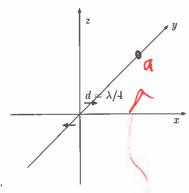
Consider a system of two x-polarized short dipoles placed on the y-axis at  $y=\pm d=\pm \lambda/4$  as shown on the left. Both dipole lengths are  $L\ll\lambda$  and both dipoles carry the same non-zero input currents except for a 180 degree phase shift, which is why the current reference directions of the dipoles are indicated by opposing arrows in the figure.
