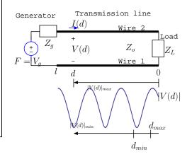
**Example 2:** If the TL circuit in Example 1 has  $l = 0.625\lambda$ , and a generator with an internal impedance  $Z_g = 50 \Omega$ , determine the generator voltage  $V_g$ .
