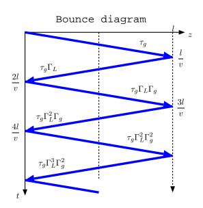
• Once the bounce diagram for voltage has been constructed as shown above, then the impulse response can be written by inspection as
