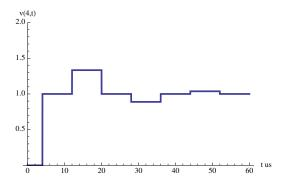
**Example 2:** In the TL circuit described in Example 1, determine V(z,t) and I(z,t) for a new source signal  $f(t) = \text{rect}(\frac{t}{T}) + 2\text{rect}(\frac{t-T}{T})$ ,  $T = 1 \mu s$ . Plot V(z,t) versus z at  $t = 3 \mu s$  and  $t = 11 \mu s$ .
