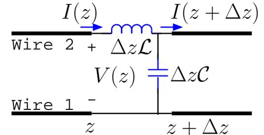
Evidently, a short section  $\Delta z$  of the TL has an equivalent T-network with
