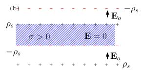
A conducting slab inserted into a region with field E\_o (as shown in b)develops surface charge which cancels out E\_o within the slab.
