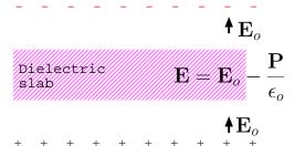
A dielectric slab inserted into a region with an initial field E\_o will become polarized.
