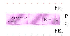
A dielectric slab inserted into a region with an initial field E\_o will become polarized.
