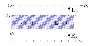
A conducting slab inserted into a region with field E\_o (as shown in b)develops surface charge which cancels out E\_o within the slab.
