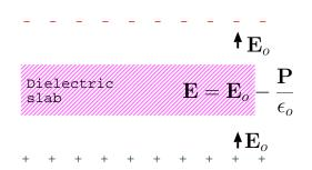
A dielectric slab inserted into a region with an initial field E\_o will become polarized.
